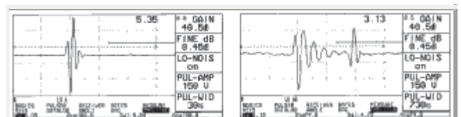
Fig. 10 a: Optimum pulse length Fig. 10 b: "Double pulse" caused by a pulser pulse which is too wide
